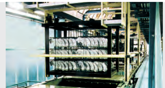
Cathodic E-coat with programmable hoist for automotive parts.
