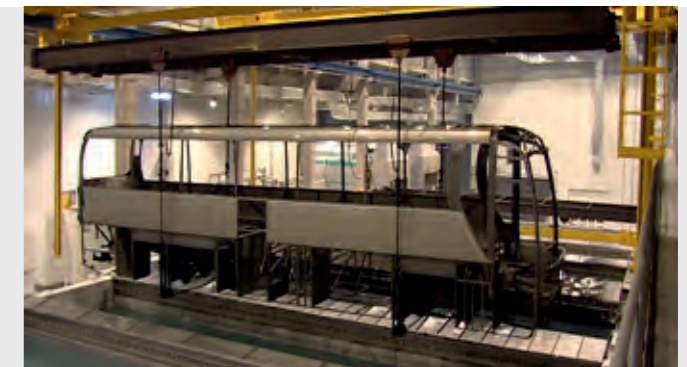
Hoist dip E-coat system for bus cabins.
