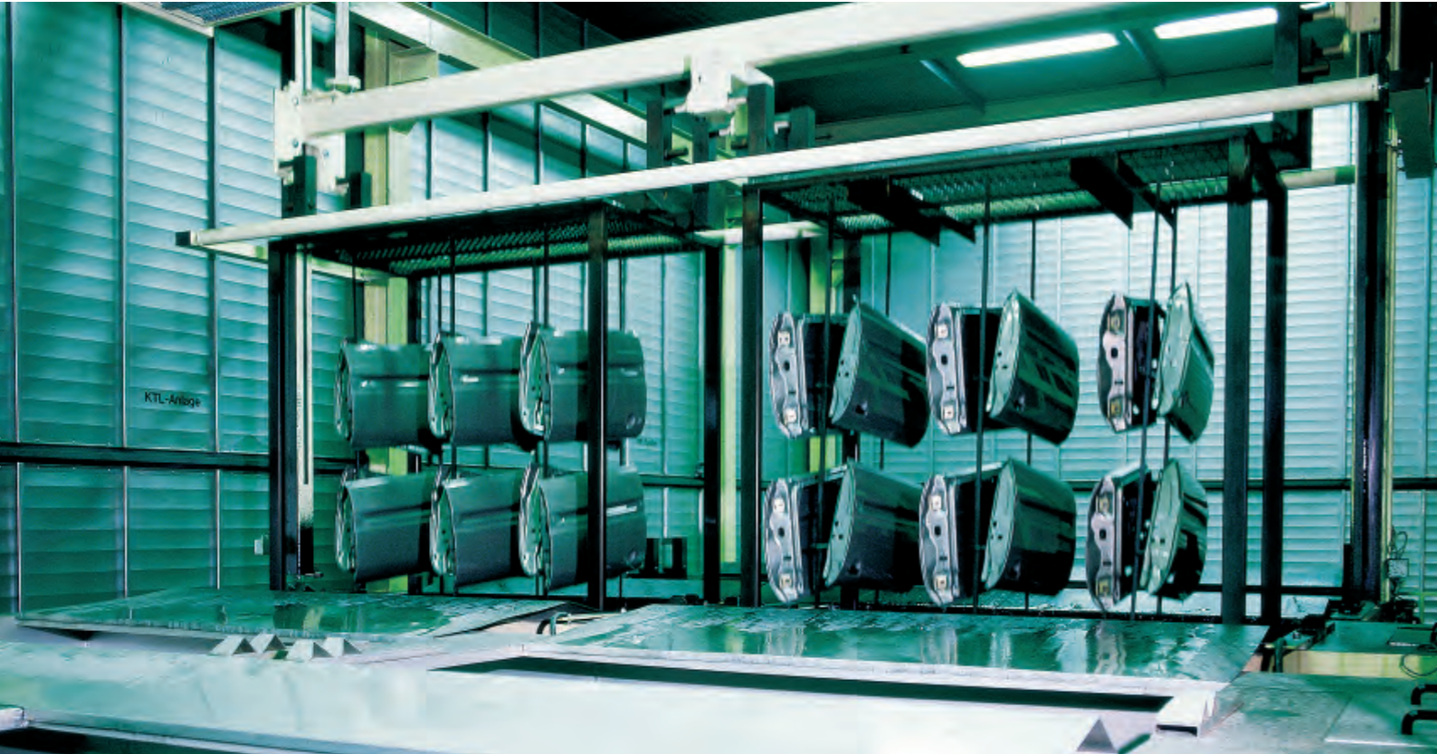
Cathodic E-coat system for automotive parts using a 10-stage pretreatment.
