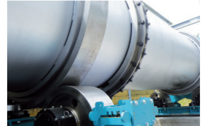
Rotary kiln for the treatment of hazardous waste.
