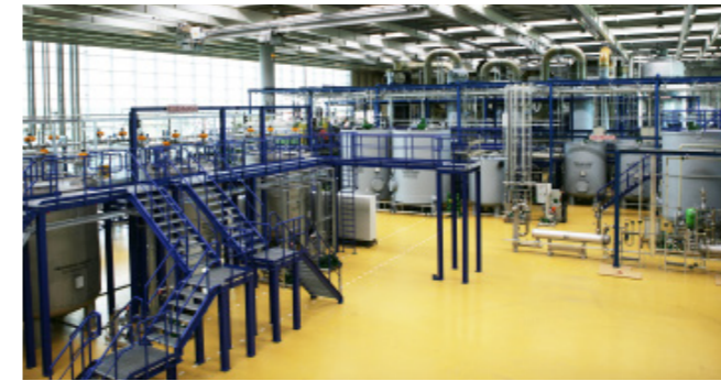
Treatment of waste water produced during flue gas purification: oxidation, precipitation, and sedimentation in a high-performance sludge settling tank.
